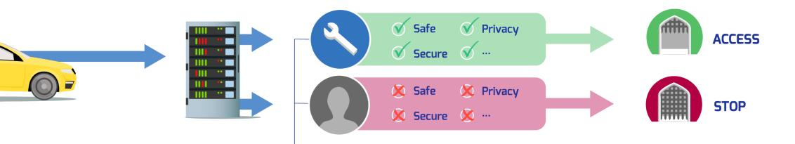
Relevant vehicle data are communicated by the manufacturer to an off-board facility Service providers can then access vehicle data through off-board means, rather than having direct access to the vehicle in an uncontrolled way The off-board facility acts as a gatekeeper, minimising safety, security and liability risks
