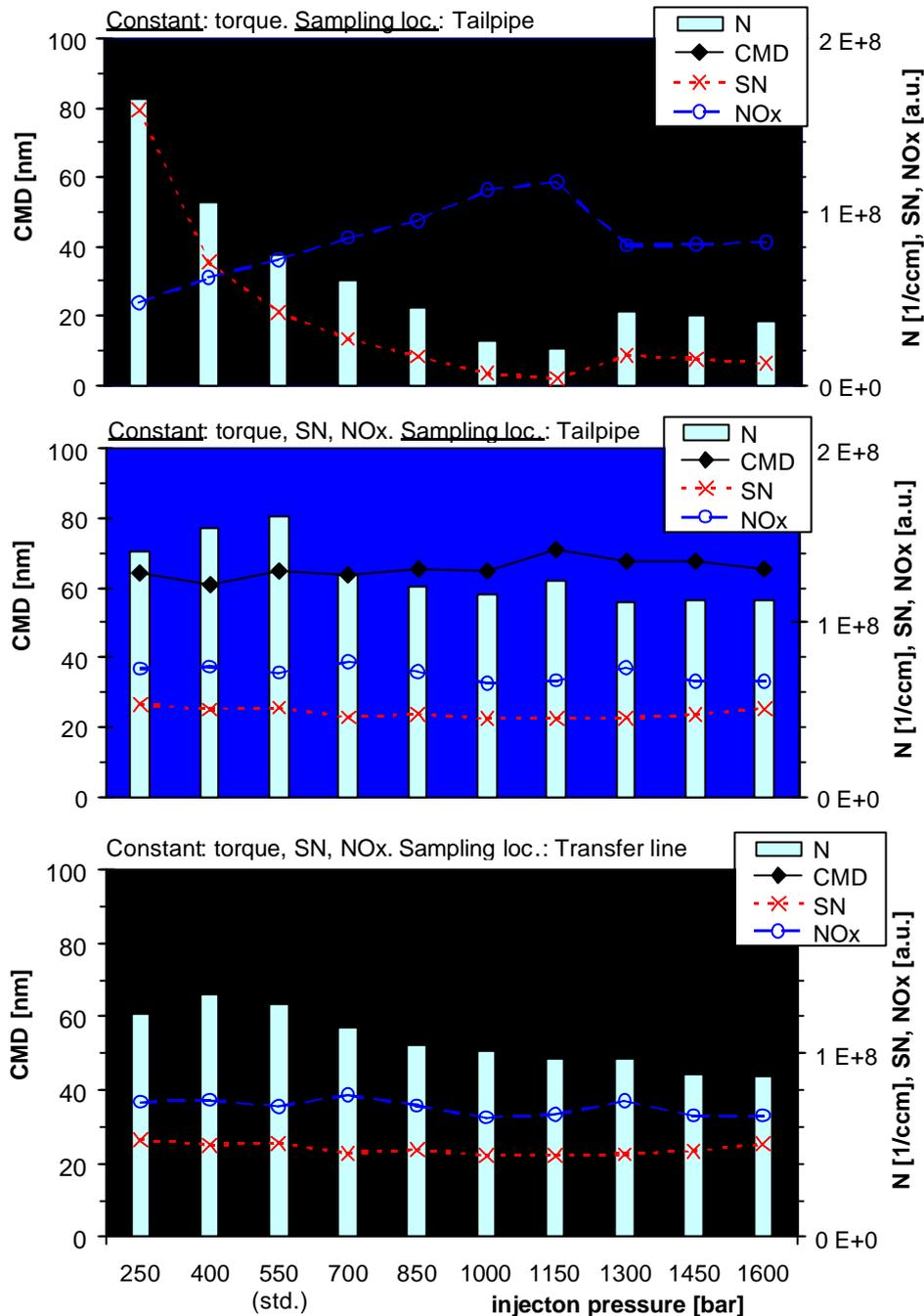
**Fig. 1:** Particle size (CMD), number concentration (N), smoke number (SN) and NOx level versus injection pressure; n = 2000 l/min, Torque = 82 Nm (v = 100 km/h). The standard injection pressure is 550 bar for this engine speed and load.
