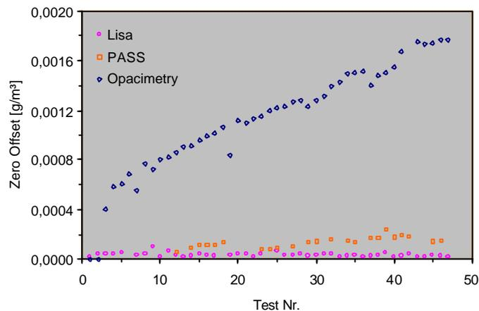
**Figure 11:** Zero drift due to fouling
