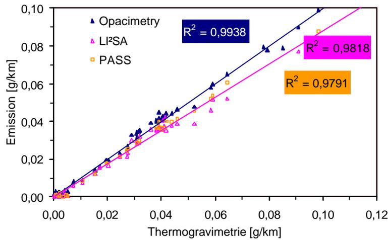
**Figure 6:** Correlation of mass emissions calculated from opacity, Li<sup>2</sup>sa and PASS with thermogravimetry (NEDC)
