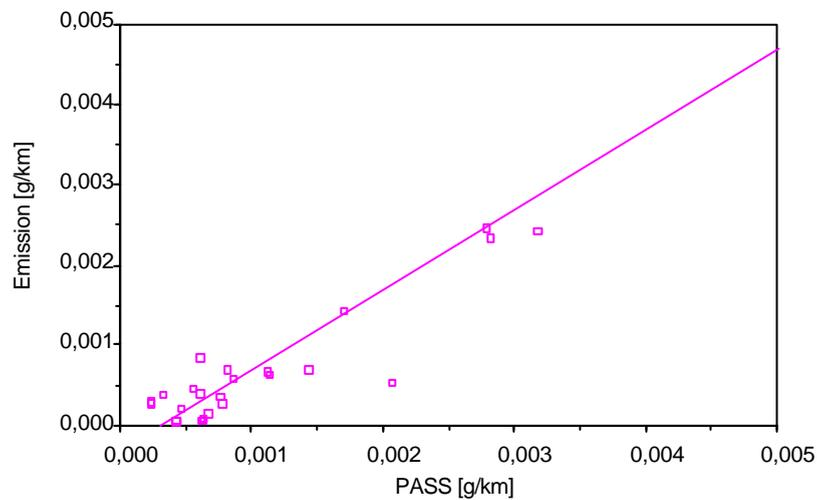
**Figure 7:** Correlation of opacity, Li<sup>2</sup>sa, thermogravimetry related mass emissions with PASS results at low emission levels
