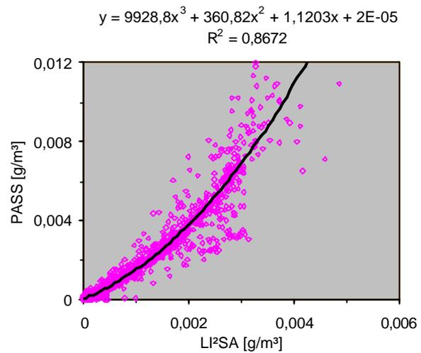
**Figure 4:** Third order calibration of Li<sup>2</sup>sa using calibrated values from PASS
