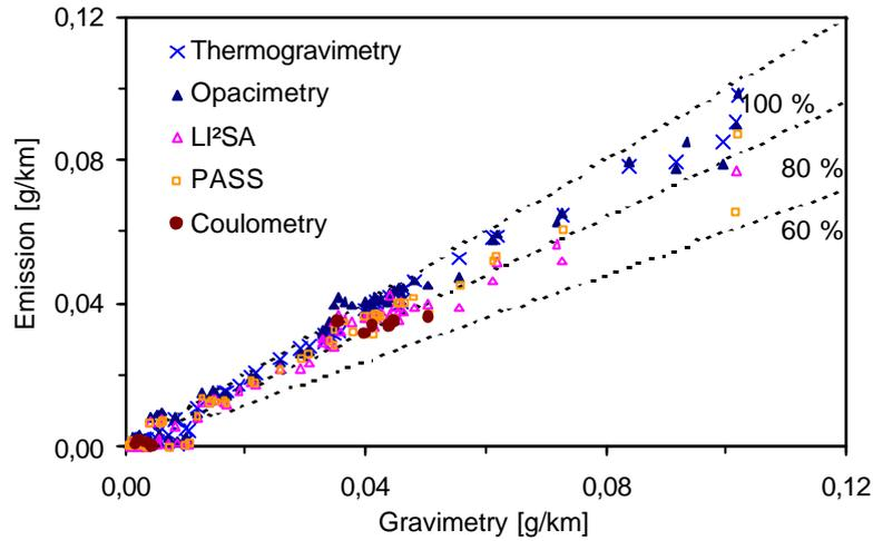
**Figure 5:** NEDC-Phase average emissions plotted over results from gravimetry
