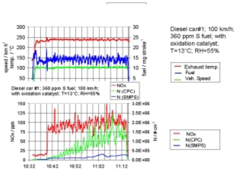
Fig. 12. Evolution of number emission (CPC and integrated SMPS) in PM size distribution during 40 min chasing at 100 km h<sup>-1</sup> and fuel consumption, exhaust temperature and vehicle speed.
