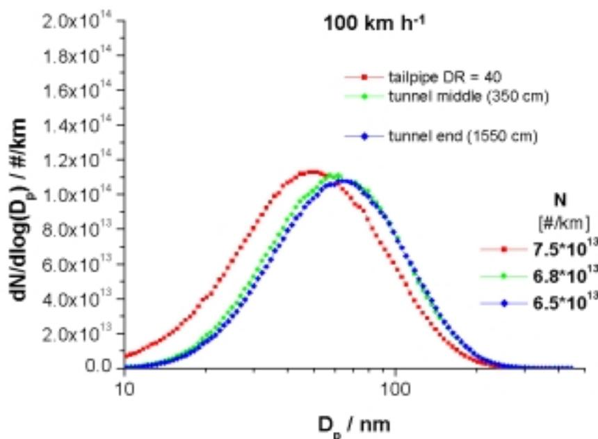
Fig. 2. Comparison of particle size distribution measured at three sampling location with the Matter diluter. The diesel vehicle was running at constant speed of  $100 \text{ km h}^{-1}$ . The Matter diluter was set to a dilution ratio of  $1:40$ . At the tunnel the total dilution ratio was  $1:440$ .
