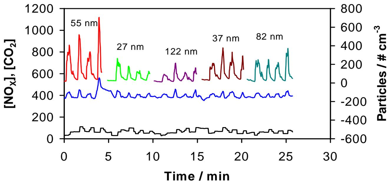
Fig. 5.  $\text{NO}_x$ ,  $\text{CO}_2$  and particles measured at a fixed SMPS size bin while drive in and out of the exhaust plume of the diesel test vehicle.
