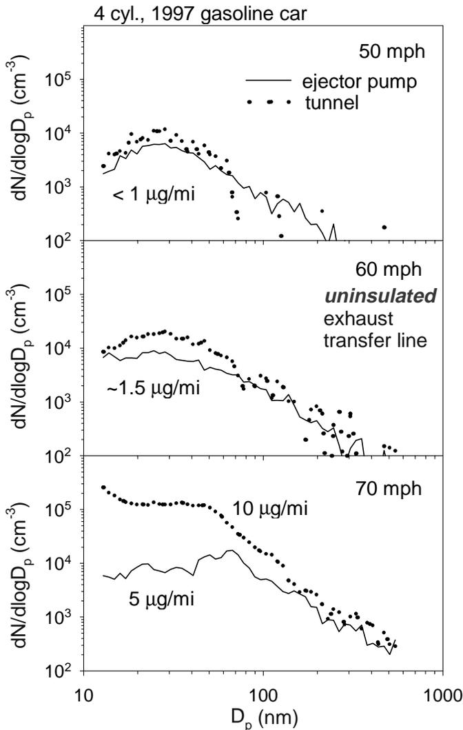
Figure 4. Comparison of ejector pump and dilution tunnel particle size distributions for the 4-cylinder, U.S., gasoline car at 50, 60, and 70 mph when using the *uninsulated/unheated* transfer line. Note logarithmic concentration axes. Mass emission rates are estimated from the size distributions.
