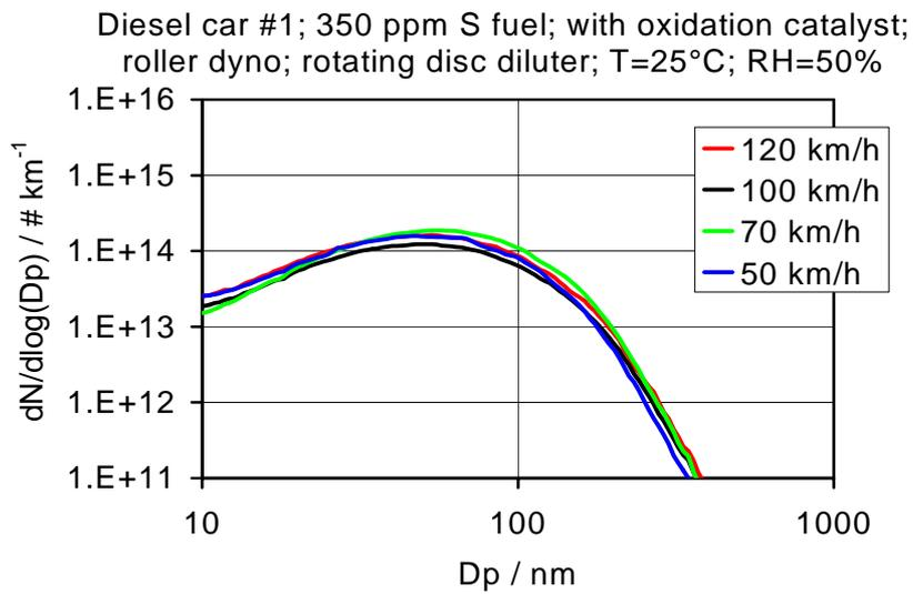
Fig. 8: Same test vehicle as Fig 7 operated at different speeds at chassis dynamometer. No nucleation mode particles were observed with rotating disc diluter.
