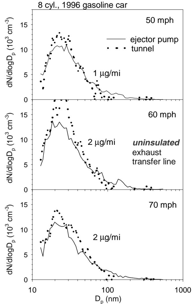
Figure 3. Comparison of ejector pump and dilution tunnel particle size distributions for the 8-cylinder gasoline car at 50, 60, and 70 mph when using the *uninsulated/unheated* transfer line. Note linear concentration axes. The tunnel background has been subtracted. Mass emission rates are estimated from the size distributions.
