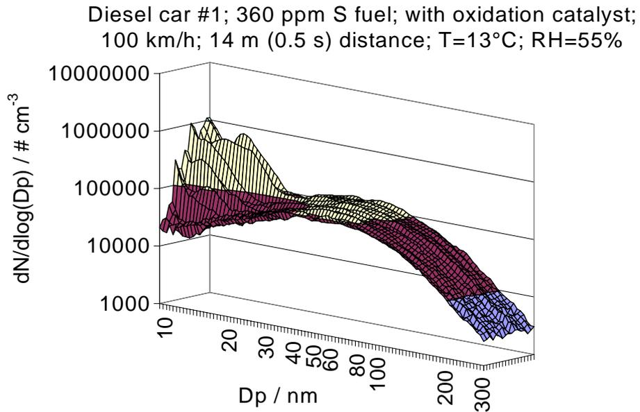
Fig. 11. Evolution of nucleation mode in PM size distribution during 40 min chasing at 100 km h<sup>-1</sup>.
