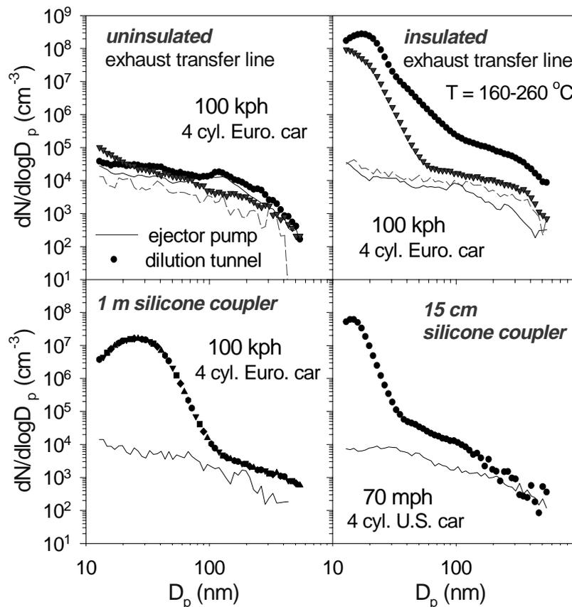
Figure 9. Comparison of particle size distributions for the 4 cylinder European gasoline car taken by ejector pump versus dilution tunnel when using a 1) *uninsulated* transfer line, 2) *insulated* transfer line, 3) *uninsulated* transfer line plus a 1 meter silicone rubber coupler, and 4) *uninsulated* transfer line plus a 15 cm silicone rubber coupler. In the top two panels, two sets of data are compared. Mass emission rates are estimated from the size distributions.
