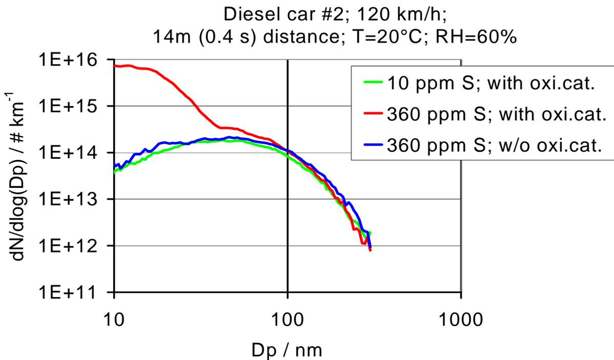
Fig. 10. PM size distributions measured in exhaust plume of test vehicle with different S fuel, with and w/o oxidation catalyst
