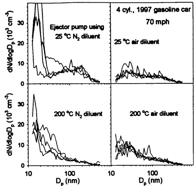
Figure 2. A comparison of ejector pump measurements of tailpipe PM concentration using N<sub>2</sub> and air diluent at either 25 °C or 200 °C. The measurements are made sequentially and are thus subject to fluctuations in the vehicle emissions.
