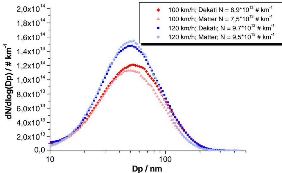
Fig. 1. Comparison of particle size distribution measured after dilution at the tailpipe of the diesel test vehicle with a rotating disk (Matter) and two ejector type (Dekati) diluters at  $100 \text{ km h}^{-1}$  and  $120 \text{ km h}^{-1}$ . The Matter diluter was set to a dilution ratio of  $\text{DR}=1:100$ ; two Dekati diluters were cascaded ( $\text{DR}=1:80$ ), connected via a reservoir volume which inserted 2 s of residence time.
