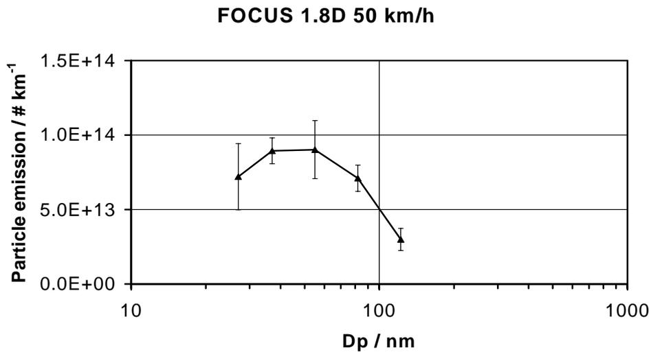
Fig. 6. Constructed size distribution from chasing experiments. The dilution ratio is calculated from the measured  $\text{NO}_x$  and  $\text{CO}_2$  concentration and the known  $\text{NO}_x$  and  $\text{CO}_2$  emission at constant speed.
