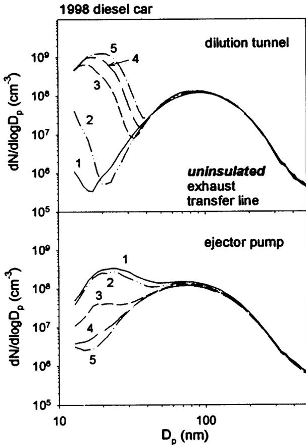
Figure 11. Sequence of size distributions taken at 3 minute intervals following an increase in vehicle speed from 50 to 60 mph. Top panel illustrates the growing in of the 20 nm artifact due to heating of the transfer hose. Bottom panel shows a transient artifact from hydrocarbon build-up that “burns off” of the j-tube sample probe in the tailpipe.
