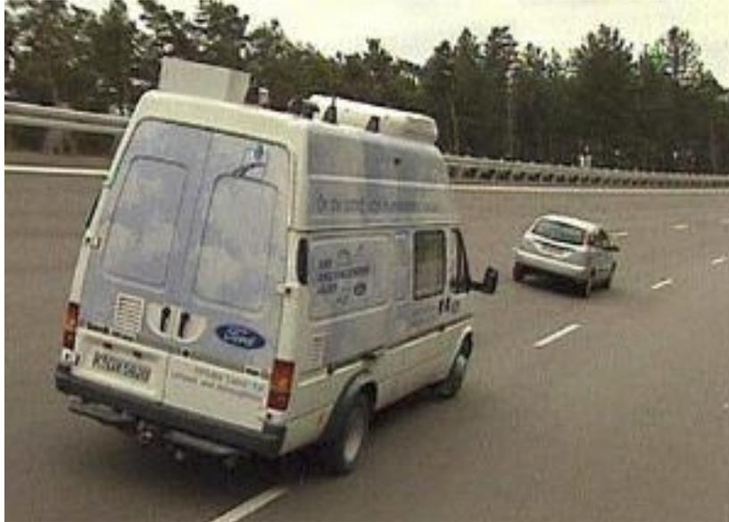
Fig. 4. Chasing of exhaust plume with Ford Mobile Laboratory
